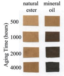
Figure 6 – 14 Kraft paper insulation after being aged in natural or mineral oil at a temperature of 150°C [145].
