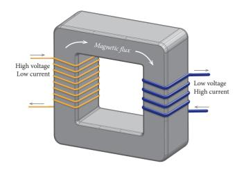
Figure 11 - 17 Principle of power transformation from high voltage to low voltage.
