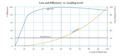
Figure 11 – 19 Losses and efficiency versus rated load of distribution transformers [181]. The load and no-load losses are indicative on this chart and describe their general function as load changes.
