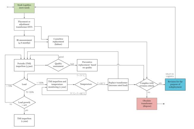
Figure 6 – 3 Flow diagram life cycle of a single distribution transformer within Liander. Adapted from the Levenloopplan Distributie Transformatoren [112]. TMI = Thermal Maximum Inspection incinerated to compensate for the energy losses. This results in the following question:
