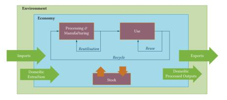
Figure 11 - 8 system scope for the comprehensive reutilisation rate [91].
