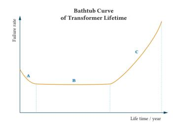
Figure 11 – 21 Bathtub curve illustrating three life cycle phases (installation, use or maintaining, and phasing out) of a distribution transformer [144].
