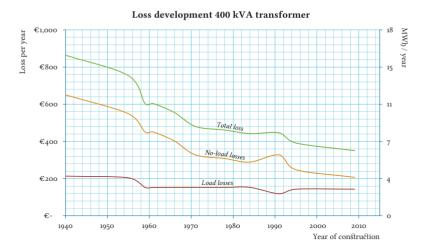
Figure 11 – 20 Historical energy loss development of 400kVA distribution transformer population operated by Liander [114]. The losses are measured at the average maximum load which is nominally at 55% of the rated load.
