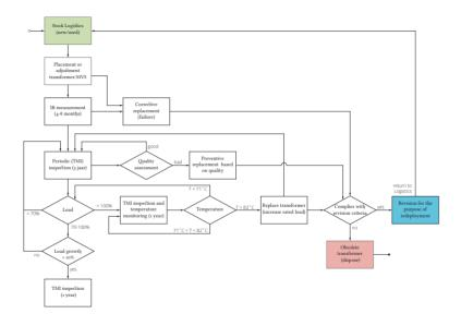
Figure 11 – 22 Life cycle guidelines for individual distribution transformer at Liander (adapted from Levensloopplan Distributie Transformatoren [112]).
