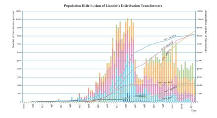
Figure 11 – 23 Current install base of distribution transformers broken down per capacity.
